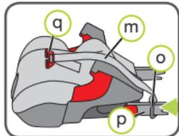
4. Place the fastening clip (q) of the flexible belt guide (m) on the surface of the booster seat.
