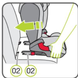
6. Place the child safety seat in driving direction on a vehicle seat approved for use. Ensure that the backrest 10 is flush with the backrest of the vehicle seat.
