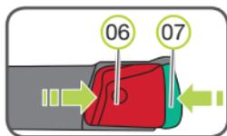
5. Push the green safety button (07) and the red release button (06) on both sides of the seat towards each other. This ensures that both hooks on the ISOFIT locking arms (05) are open and ready to use.
