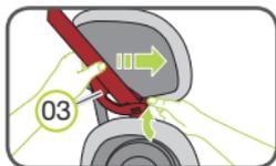
1. Press the release button of your vehicle seat buckle and guide the safety belt back.
