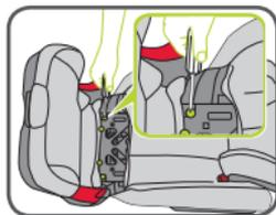
4. Release the 4 Torx screws on the backrest (12).
