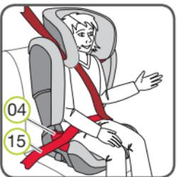
6. Also place the lap belt section (15) on the other side of the seat cushion in the bright red belt guide (04).
