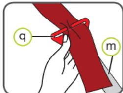
6. Mount the fastening clip (q) on the diagonal seat belt section. Ensure that the belt of the flexible belt guide (m) is not twisted.
