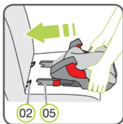
4. Place the child safety seat in driving direction on a vehicle seat approved for use. Ensure that the backrest 10 is flush with the backrest of the vehicle seat.
