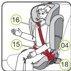
5. Place the diagonal seat belt section (16) and lap belt section (15) on the side of the vehicle seat belt buckle (18) into the bright red belt guide (04) of the seat cushion.
