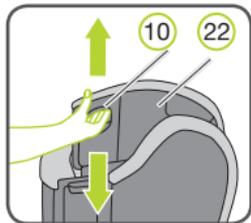
1. Reach into the adjustment handle (10) on the back of the headrest (22) and pull it towards you. This unlocks the headrest.
