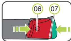
3. Push the green safety button (07) and the red release button (06) on both sides of the seat towards each other. This ensures that both hooks on the ISOFIT locking arms (05) are open and ready to use.
