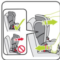
10. Shake the child safety seat to ensure that it is securely fastened and check the fastening buttons again 07 to ensure that **both** are fully green.
