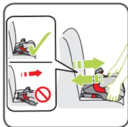
8. Shake the child safety seat to ensure that it is securely fastened and check the fastening buttons again 07 to ensure that **both** are fully green.
