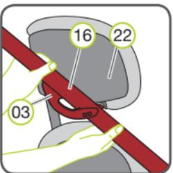
7. Guide the diagonal seat belt section (16) into the dark red belt holder (03) of the headrest (22) until it lies completely inside the belt holder (03) and is not twisted.
