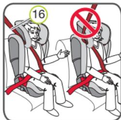
**DANGER!** The diagonal seat belt section 16 must never lead forward to the vehicle's belt deflector. In this case, only use the vehicle child seat on the rear seat.
